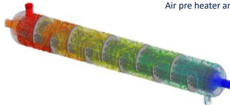
Thermal analysis of Shell & tube heat exchanger
